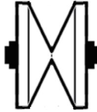
Fig. 4. Modified wheel of modified transplanter takes the cross soil furrow shape
