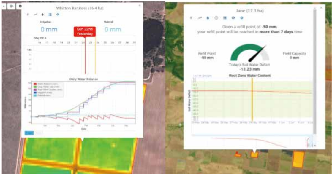
그림 4 | Irrigation scheduling information and forecasted irrigation deficits for the coming 7 days shown in IrriSAT
